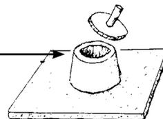
To make the **closed latrine**, the slab should be placed over a round hole in the ground. Dig the hole a little less than 1 meter across and between 1 and 2 meters deep. To be safe, the latrine should be at least 20 meters from all houses, wells, springs, rivers or streams. If it is anywhere near where people go for water, be sure to put the latrine **downstream**.
