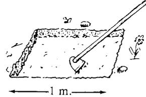
2. Make or cut a wire mesh or grid 1 meter square. The wires can be ¼ to ½ cm. thick and about 10 cm. apart. Cut a hole about 25 cm. across in the middle of the grid.
