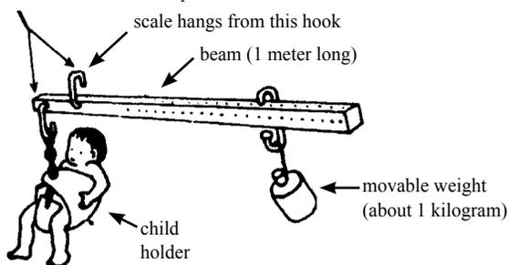
Weight is correct when beam stays horizontal.
