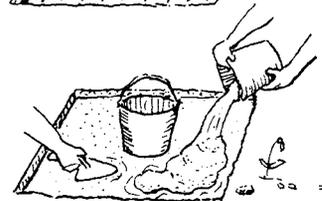
6. Remove the bucket when the cement is beginning to get hard (about 3 hours). Then cover the cement with damp cloths, sand, hay, or a sheet of plastic and keep it wet. Remove the slab after 3 days.
