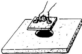
Keep your latrine clean. Wash the slab often. Be sure the hole in the slab has a cover and that the cover is kept in place. A simple cover can be made of wood.
